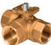
Ball valves designed for control of hot, cold or glycol-mixed water in heating and ventilation systems. These ball valves can be used as either characterized control ball valves when a flow plate is installed in port A (default mode), or as on/off ball valves when the flow plate is removed. When the flow plate is removed the Kvs between port A and AB is increased. The valves are intended for use with Regin's RVAB4/RVAB5 actuators.
