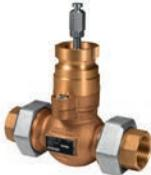
ETVS: 2-way control valves, DN15-50, kvs 0.25-40, 20 mm stroke, DZR
