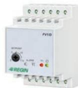
The electronic frost protection unit is mainly intended for use in air handling systems. If the temperature falls below the setpoint, the relays will fall and an alarm LED lights up. The unit should be connected to an NTC sensor placed on the heating coil or return water pipe. The frost protection unit has two alarm relays and manual or automatic reset. The sensor must have 0...30°C temperature range.
