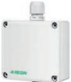
This device measures the carbon monoxide concentration using an electrochemical method of measurement characterised by high selectivity even in low concentrations. It is installed for both safety and energy-saving reasons. The output signals are linear representations of the gas concentration.
