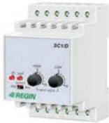
Step controller suitable for heating/cooling or alarm applications. It converts a 0...10 V DC input signal to a relay output. The controller is suitable for DIN-rail or cabinet mounting and have adjustable switching points. The step controller with 2 relays can be set to either binary or sequential control. Individually settable on/off levels.
